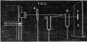
mirror on fork C, and thence to the screen. When the forks vibrated in unison a luminous band, D E, appeared. When one, as the lecturer expressed it, was "jockeyed" with the weight of a cent, the band alternately shortened and lengthened. By reflecting this from a looking glass, as before, the sinuosities on the screen appeared as in Fig. 6, their differ-
