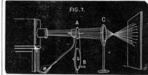
vibrations due to a sound may be determined. Passing the light through the cylinder and lens, the perforations appeared on the screen as shown. Then by forcing in air and rapidly revolving the disk, producing a dismal species of caterwaul, the lecturer reflected the luminous dots on the screen from a hand mirror. On vibrating the latter the most curious undulatory sinuosities appeared-circles interwoven with each other wonderfully intricately, besides other singular combinations of form.
