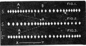
the rarefied wave. In Fig. 3 this same particle has returned to its former position. It has consequently made an excursion to and fro over the length, X Y, oscillating, in other higher the pitch of the note. By this means any number of words, throughout this distance.
