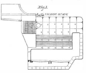
heating tubes. The steam passes from the boiler into the superheater and thence to the engine in the usual manner. We also give a diagram on an enlarged scale of the upper portion of the boiler and superheater at the junction with the uptake. It was at the corner  $\Lambda$ , where the uptake begins, that the felting took fire, and the ignition was occasioned by
