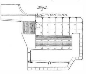
heating tubes. The steam passes from the boiler into the superheater and thence to the engine in the usual manner. We also give a diagram on an enlarged scale of the upper portion of the boiler and superheater at the junction with the uptake. It was at the corner A, where the uptake begins, that the felting took fire, and the ignition was occasioned by
