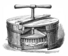
ing. The device consists in a tub or bex, the bottom of which is made corrugated. A circular brush fits loosely within the tub, and is movable by the lever handle represented. A close fitting cover, held down by a bar and loops, covers the receptacle. The clothes are thoroughly washed by placing them between the brush and corrugated bottom, and retating the former.
