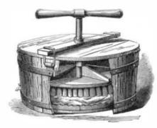
ing. The device consists in a tub or bex, the bottom of which is made corrugated. A circular brush fits loosely within the tub, and is movable by the lever handle represented. A close fitting cover, held down by a bar and loops, covers the receptacle. The clothes are thoroughly washed by placing them between the brush and corrugated bottom, and rotating the former,
