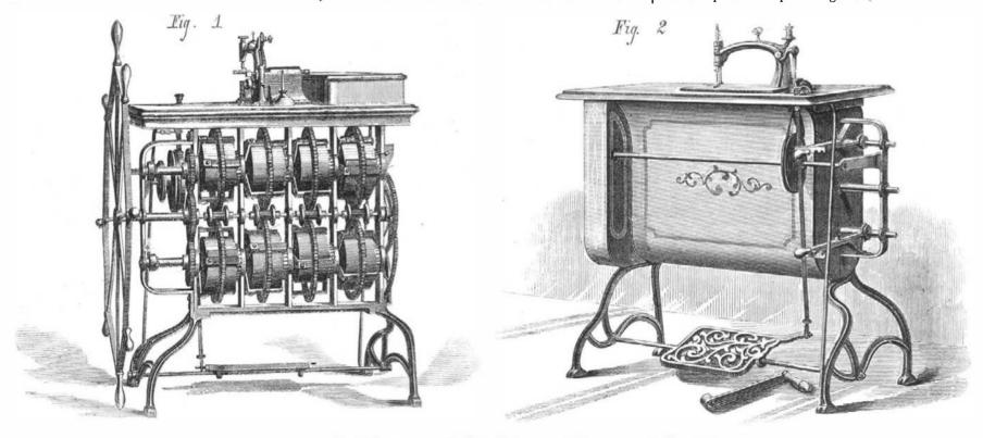
The invention we now illustrate appears to meet the re quirements of the case by furnishing a simple and economic motor which can conveniently be applied to any form of the sewing machine. It consists of a spring power, mounted in a neat frame, to the top of which the table of the machine is attached.
