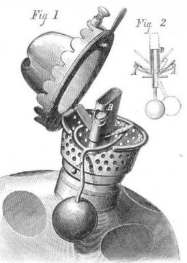
In the provision thus made for extinguishing the lights before the oil in the lamp has time to escape and become ignited, appears to lie a safeguard against many of the disastrous results hitherto attending lamp accidents.
