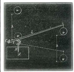
Let h represent the vertical hight which the weight, w, moved, and d the distance which the nail was driven into the wood. Then
