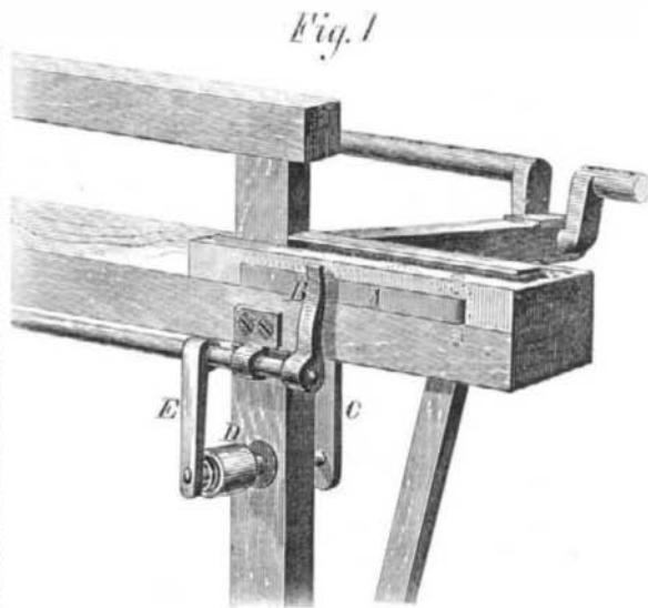
Fig. 1 represents a portion of the lathe of a loom, showing part of one sword, one rod connecting the lathe with the crank, and the device attached. Fig. 2 is a detail sectional view of the same.
