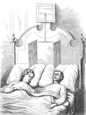
head of a bedstead and employed to swing a double fan for the two fold purpose of cooling the air and keeping off files and mosquitoes. The inventor states that the machine, when actuated by a weight, will run for six hours and a half where the room is ten feet high. He considers the employment of such a fan in the sick room most advantageous.
