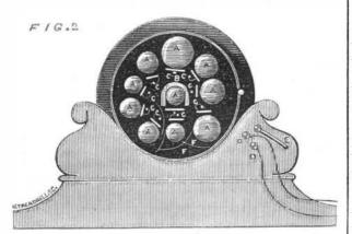
face of the barometer. To effect this closing of the circuit the face of the barometer is provided with a series of platinum conducting pins, and whenever, by a change in the atmospheric conditions, the pointer is moved it touches a corresponding pin, and the bell that is in connection with such pin is sounded.
