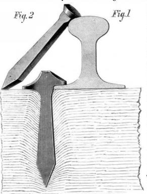
chair spike, Fig. 2, is made with a round head, and, being otherwise constructed on a similar principle to that above described, it possesses the same advantages. The practical utility of the invention is plainly evident, and as its expense is necessarily no greater, it will doubtless be preferred to the straight and less effective spike now in use.
