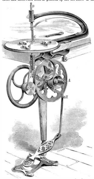
Around the circumference of the wheel, A, is placed a covering of leather, by the friction of which the pulley, B, and the fly wheel connected therewith are actuated. By means of the pitman, as shown, motion is transmitted to the saw. G is an adjustable metal foot designed for holding the work in place while being operated upon.
