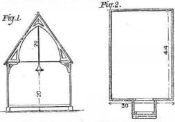
out any arch to the cciling; then break it up by showing the principal trusses (three in number) extending across the roof. It is best to make these simply to consist of the two rafters and a short hammer beam at bottom on each side, and, in the absence of buttresses, connect these by a 1½ inch iron tie rod. At the center of each tie rod, bring a rod down from the ridge to support the chandellers, with an ornamentat the intersection of the two.
