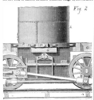
clearly in Fig. 3. D is the outer transient ring in which are placed eight metallic cylindrical rollers, E E, held with their axes vertical. These project beyond the inner surface of the ring. D. and impinge upon the inner transient ring. C. so as to admit of the rotation of the former around the latter. Two trunnions, F F, on either side serve to support the ring, D, and at the same time allow it to freely oscillate in the bearings on the car frame, G. H, Fig. 2, is one of the
