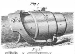
a stirrup, in two pieces, which are halved together as shown and joined by screws at the point, F. Its fulcrum pins are represented at G, on the male part of the coupling, while the cam hooks, H, in which the short ends of the lever terminate, engage the fastening pins, J, on the female portion.
