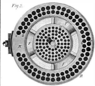
surrounding casings of the mixing chamber, and finally cov er the lower portion of the steam drum, this central chamber adds greatly to the already large separating surface, so that steam may be rapidly disengaged without carrying up water into the steam pipes.
