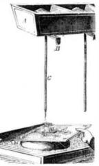
As fast as the supply of engraving powder runs down through the tube, it is replaced in the hopper; and girls may do all the work. That portion of the articles that is not to be engraved is protected by paper or other substance. The engraving, therefore, is done by cutting out the desired pattern in paper, which is then applied to the surface of the article. The powder only acts between the interstices of the pattern.
