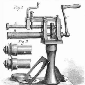
are two shafts which carry the cutters. The top one, A, is adjustable, by means of screws, to any required distance from
