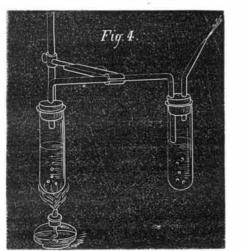
ture. I put in action. You see that in this space of time but a very small quantity of water has distilled; but look at the worm tub, and you see that a large quantity of water which was ice cold at starting has been made itself to steam-by what? By the heat which that small quantity of water contained when it was steam.
