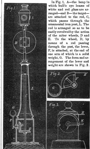
Fig. 3 represents the signal post, on the exterior of which is a hand lever, K, working in a semicircular guide and tnrning the sheave, J, within the post. 'To the circumference of this sheave, the wire, H, is fastened, passing therefrom over other sheaves for a distance of from 1,000 to 2,000 feet, until it reaches the lever, described on Fig. 1, to which it is attached, as shown on Fig. 2.
