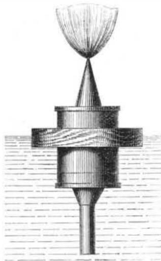
The apparatus, an invention of N. T. Holmes, consists of a sheet metal cylinder, having a conical top and a tube of about six inches in length projecting from its bottom. It is filled with phosphate of calcium, which is prepared in the following manner: Pieces of chalk are put into a crucible, together with a quantity of amorphous phosphorus, and then brought to a white heat. The chalk, becoming incandescent, absorbs the vapors of phosphorus, and thereby becomes phosphate of
