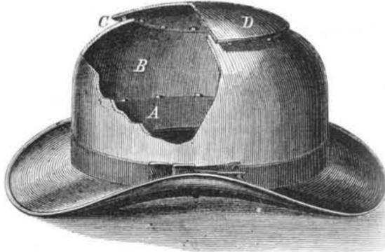
The making of a few perforations at the top of the crown of a hat does not really make a ventilating hat. To ventilate an air space requires either very much larger openings than these, in proportion to the space to be ventilated, or else openings below as well as above, so that the currents of heated air rising may meet opposing descending currents, and may be freely replaced by cooler air entering at the bottom.
