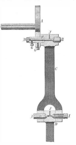
working loose of the parts. The construction obviates th jar consequent upon loose connections, a.d also affords ease in repairing, providing for ample and continuous lubrication and protection of the bearing parts from grit and dust.
