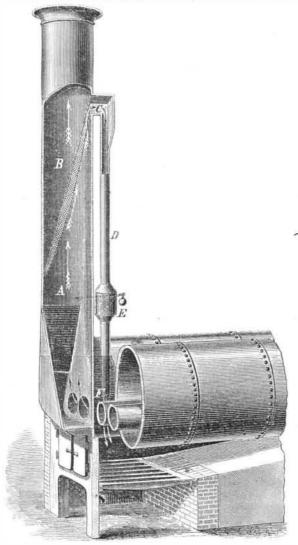
form to correspond with the section of the uptake made at the same angle. While the smoke and gases of combustion pass freely through it, it stops the sparks, which are directed by the upward current along its under inclined surface through the opening, C, into the flue. D, leading downward to the fire box. Faliing upon a counterpoised valve, E, they accumulate till they are dropped, through F, into the fire box, where they are consumed.
