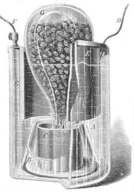
If, just previous to this period, the flask be removed and supplied with sulphate of copper crystals, enough of the solution of the latter will remain in the cup, B, to maintain the action of the battery during the process of filling, so that the duration of the action is practically limited only by the consumption of the zinc.
