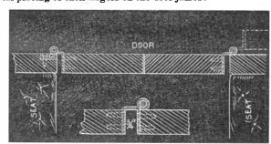
It is to leave a space of three fourths of an inch between the door and the frame, so that it would be impossible for the door to tighten upon the fingers, should they be in the space. This might be done in existing carriages by cutting away the frame, or reducing the door, or both; but best of all by a new door made narrower than the doorway.
