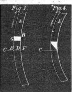
In Fig. 4, it will be seen that the back of the piston is sloped off at such a rate as If we also slope off the abutment and make it very thick, we may virtually get rid of the clearance difficulty altogether. It may, therefore, be laid down as a principle that it is possible so to shape an abutment working vertically and a piston working circum-
