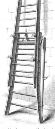
The roller, B, is turned by the crank, C, either directly or by means of a rod or pitman, D, by the use of which the roller may be turned and the ladder extended by a person standing upon the ground, so that a person standing on the movable part may be raised or lowered, to the hight required, by those below. A self-acting brace, E, holds the parts extended in any required position.
