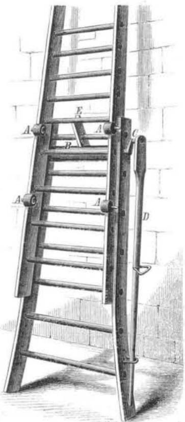
The roller, B, is turned by the crank, C, either directly or by means of a rod or pitman, D, by the use of which the roller may be turned and the ladder extended by a person standing upon the ground, so that a person standing on the movable part may be raised or lowered, to the height required, by those below. A self-acting brace, E, holds the parts extended in any required position.
