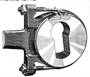
The eccentric strap, B, extends from two lugs formed on the connecting rod about the eccentric, A, as shown, the ends of the strap passing through the lugs and being threaded to receive the tightening nuts.
