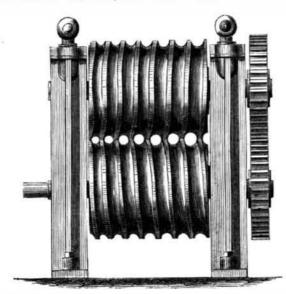
gether and geared, so as to revolve in union, the grooves form a series of eyes, which, as the rolls revolve, appear to move laterally, and gradually decrease in size. Thus, if a bar or tapered strip of iron, bent so as to approximately form a tube, be introduced between the rolls at that end where the grooves are largest and deepest, it will be gradually shifted towards the other end of the rolls as it passes between the latter, and will thus be rolled tapered.
