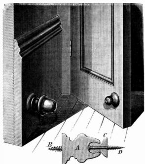
thrown open, and at the same time to keep the doors in the open position when so desired. The objection to devices now in use, for overcoming the concussion in throwing the door against the washboard pedestal, is the rebound they give the door, throwing it away from the position designed for it. To obviate this, several devices have been brought out, consisting of springs, ratchets, catches, etc., most of which have been proved too intricate and expensive for the purpose.
