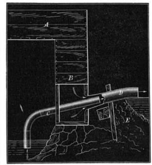
through your columns for the benefit of "our" mechanical family. Millwrights often work at a great disadvantage from the difficulty and expense of removing the water from the foundations of their mills during construction; this de vice will in many cases remove that difficulty at a very small cost. The whole thing can be made by any good carpenter with a few planks and pieces of stove pipe.
