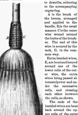
The braided wires thus hold and bind the coils, so that should the tack, D, work out, or any part of the outer wires be broken, the brush is firmly held. Four, more or less, of the braided wires may be used as deemed convenient and tasteful.
