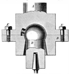
work. It requires no adjustment to center, being so con structed that the point of the drill may be placed upon the point desired to be drilled, where it will remain.
