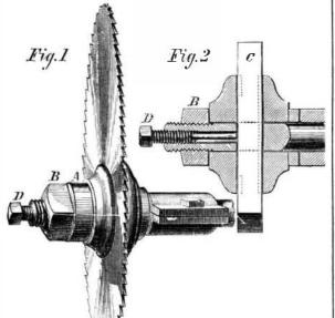
D. Then the loose collar, being placed against it, the nut, B, is firmly turned down, clamping the tool securely.
