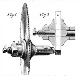
D. Then the loose collar, being placed against it, the nut, B, is firmly turned down, clamping the tool securely.
