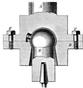
work. It requires no adjustment to center, being so con structed that the point of the drill may be placed upon the point desired to be drilled, where it will remain.
