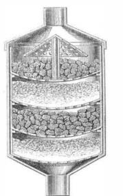
N.Y. It consists in a series of pans arranged one above the other, in the manner shown, in a suitable receptacle. Char coal and gravel may be used as filtering material, or any other approved material found convenient may be substituted. The water entering the filter falls upon a perforated 'cone, which distributes it over the filtering material in the upper pan. It then passes through the substances placed in the lower pans, and is drawn off free from impurities at the living. bottom.
