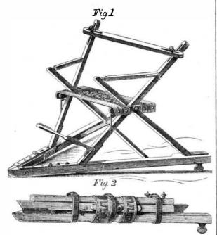
The seat is flexible, and may be made wide enough to accommodate two or more persons. A convenient support for the feet is also provided, as shown in the principal figure in the engraving, representing the velocipede in readiness for
