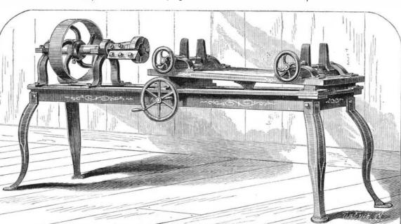
MACHINE FOR TURNING THE ENDS OF AXLETREES,
