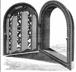
each lower corner and one at the middle of the arch at the top, as shown. This allows the front molding and register to be attached after the plastering and painting is done in new buildings, so that its finish is not marred by droppings cleaning. The application of these improvements does not while the rear corners run either on skate runners or rollers are raised, and the slabs of compressed clay are thrown out affect the general ornamental design of such registers. Pat-
