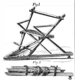
The seat is flexible, and may be made wide enough to accommodate two or more persons. A convenient support for the feet is also provided, as shown in the principal figure in the engraving, representing the velocipede in readiness for
