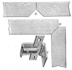
the hinges over those of the old style is trifling, and the bevel can be worked and the hinge put on, thereby completing the joint, in a very few minutes, by any ordinary mechanic. The positions of the joint when the leaf is dropped and extended are respectively shown at D and E.
