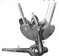
The part. A. screws into the end of the neck voke, in the usual manner. The ring, B, is made of an elongated angular shape, as shown, and has pivoted to it, at C, a slide, D. This slide is made with a broad surface, upon which the breast strap draws; the method of pivoting allowing any ordinary motion of the ring to take place without any sliding of the strap on the ring and consequent wear. The strap is, more over, kept smooth and flat on the slide, which also adds to
