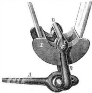
The part, A, screws into the end of the neck yoke, in the usual manner. The ring, B, is made of an elongated angular shape, as shown, and has pivoted to it, at C, a slide, D. This slide is made with a broad surface, upon which the breast strap draws; the method of pivoting allowing any ordinary motion of the ring to take place without any sliding of the strap on the ring and consequent wear. The strap is, moreover, kept smooth and flat on the slide, which also adds to its durability.
