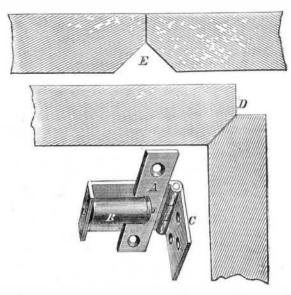
the hinges over those of the old style is trifling, and the bevel can be worked and the hinge put on, thereby completing the joint, in a very few minutes, by any ordinary mechanic. The positions of the joint when the leaf is dropped and extended are respectively shown at D and E.
