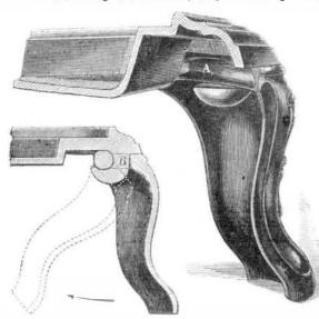
position shown in dotted outline in the sectional detail. This requires the raising of the stove bodily from the floor an inch and one half or two inches. In no other way can the leg be loosened. So long as the stove rests upon it, it cannot be moved in any direction.
