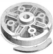
The parts are all accessible for inspection, the weight is supported independently of the packing, the packing automatically adjusts itself to any slight taper there may chance to be in the bore of large cylinders, in the bore consequent upon strain, springing, or other causes; and and this self-adjust-
