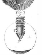
firmly against the seats. A rocking motion of the stema will then polish down the valve seats to a perfect joint. The valve disks are readily ground by placing a piece of fine emery cloth on a piece of planed iron and rubbing the
