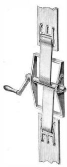
This instrument will be found of great service in bringing together the ends of belts, the weight of which is so great that they cannot be held together by the hand while lacing. A strap engages with holes made in the belt, at the back of the holes punched for lacing, the tightening strap being provided with claws or hooks, as shown. A winch axle and ratchet, adjusted in a frame as shown, are then employed to pull the ends of the belt together and hold them firmly till the lacing is completed.
