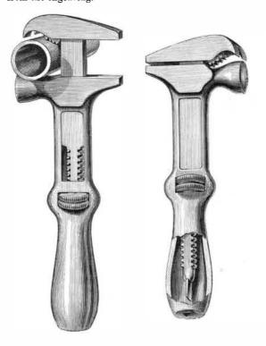
The tool is very compact, and has this advantage over the ordinary screw wrench, that its leverage increases as it is opened to receive nuts of larger size.
