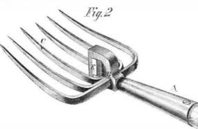
At the lower end of the handle, A, is formed a head, B, as shown, having an L-shaped slot. The tines, C, are made in pairs; each pair being united in the form of the letter U, but each successive interior pair forming a narrower U than the next pair exterior to it.
