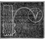
employed: A bent steel spring bar, having a Vshaped bearing, in which one of the journals of the cylinder to be balanced rests; the other end rests in a bearing adjustable vertically, so that the cylinder may be brought into a horizontal position. This being accomplished, the cylinder
