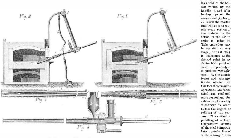
to test the degree of refining of the cast iren. This method of puddling at a high temperature admits of the steel being run into ingots in lieu of withdrawing it from the furnace in blooms as in ordinary pud-
