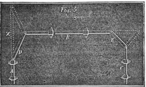
up to the point x, and the bars, B and E, will take the position shown by the broken lines on the right. The bar, C, will have made one whole reciprocation. Continue the motion of A to the position shown by the broken lines on the left; C will then have made two reciprocations. Move A back to its original position, and C will have made four reciprocations, while A has made but one. This beautiful link motion is the invention of the author of the movement shown in Figs. 3 and 4.
