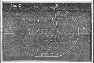
it the wiper, C; this successively engaging with the pins, D, E, F, G, imparts the motion required, the number of intermissions being varied with the number of pins. I have made a model of this movement, and it works in all respects as described.
