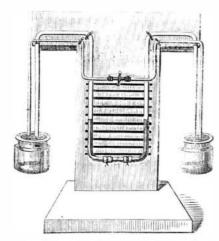
tinct horizontal lines. The hight of the apparatus is 1 foot 7 inches; the greatest width, 1 foot. Two-ounce bottles are used for the air vessels, and they are supported at the hight of about 5 inches from the ground, the main tubes rising 10 inches above the corks.
