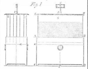
which the liquid to be evaporated is poured, until it reaches a, a.. In the middle of the box a rod, E F, passes, this rod is
