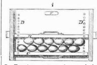
and bottom, provided with boards, BC, arranged to be moved up and down and secured at any point within by running the rods, E, through the holes, D, and through holes bored in the ends of the boards, B
